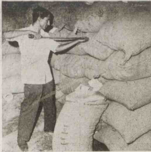
FIG. 50—Bag triers can be inserted carefully between the threads of gunny bags without breaking them when sampling.
