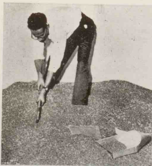
FIG. 49—A long double tube trier is useful when sampling heaps of uncleaned seed.
