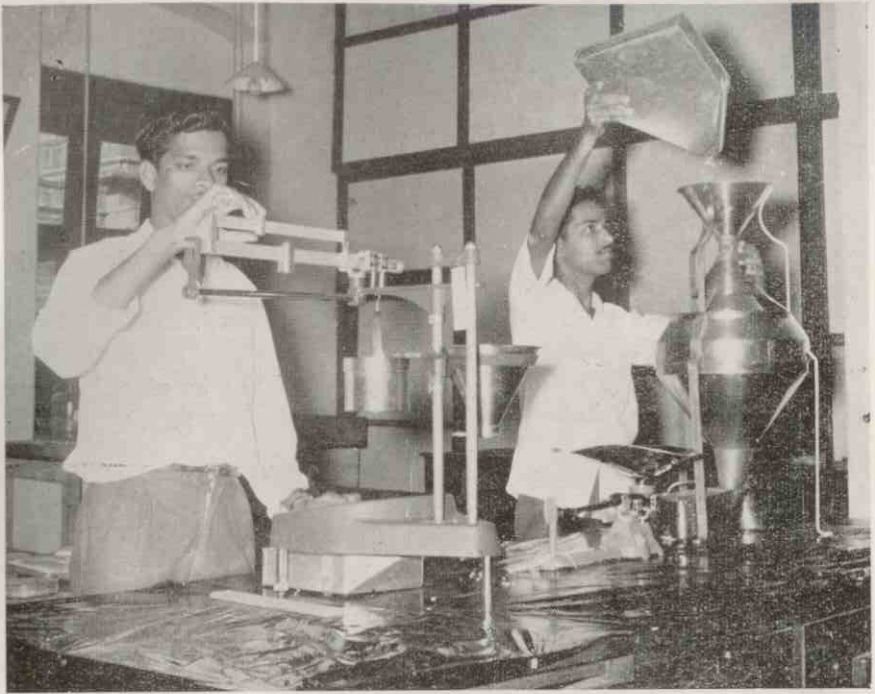
FIG. 52—Most laboratories provide a special place for entering samples and mixing and dividing them in a mechanical divider. The measure weight may also be taken at this point.
